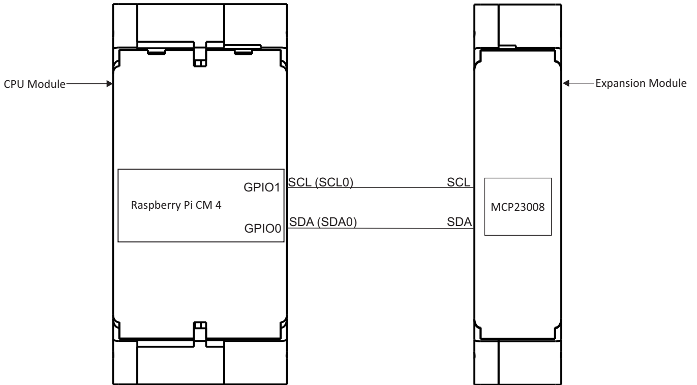
Figure 6: The GPIO connection with CPU module and Expansion Module.
